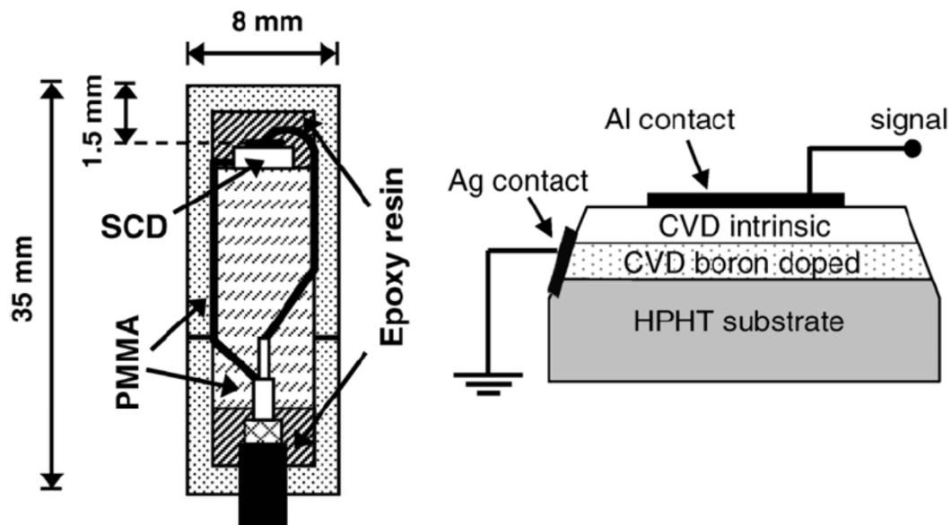
Schematic diagram of the SCD dosimeter showing longitudinal cross-section (left) and details of connections (right)
