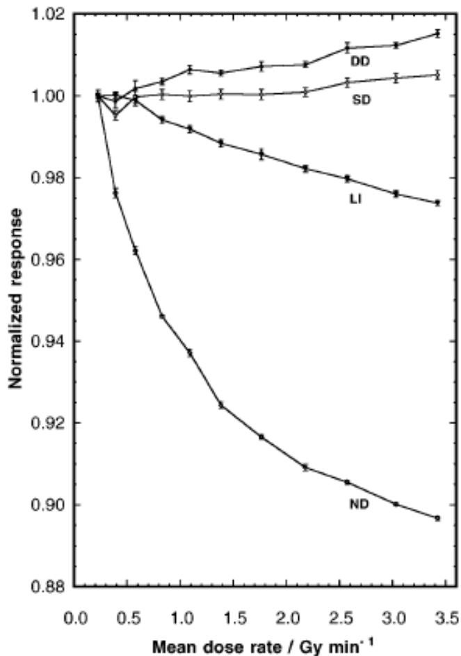
**Dose rate dependence for various detectors for 6 MV irradiations – data normalized to Farmer chamber**
