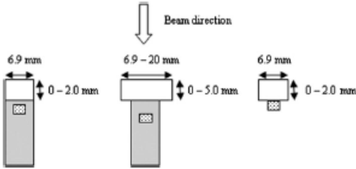
**Figure 1.** Schematic of the placement of the air gap proximal to the diode detector. The grey represents the body of the detector, the dotted area is the silicon chip, and the white is the air gap. From left to right are schematics of the PTW60017 diode, PTW60016 diode and the unenclosed silicon chip respectively. The geometry of both the air gap and the detector is cylindrical in the perpendicular to beam direction. The diagram is not to scale.
