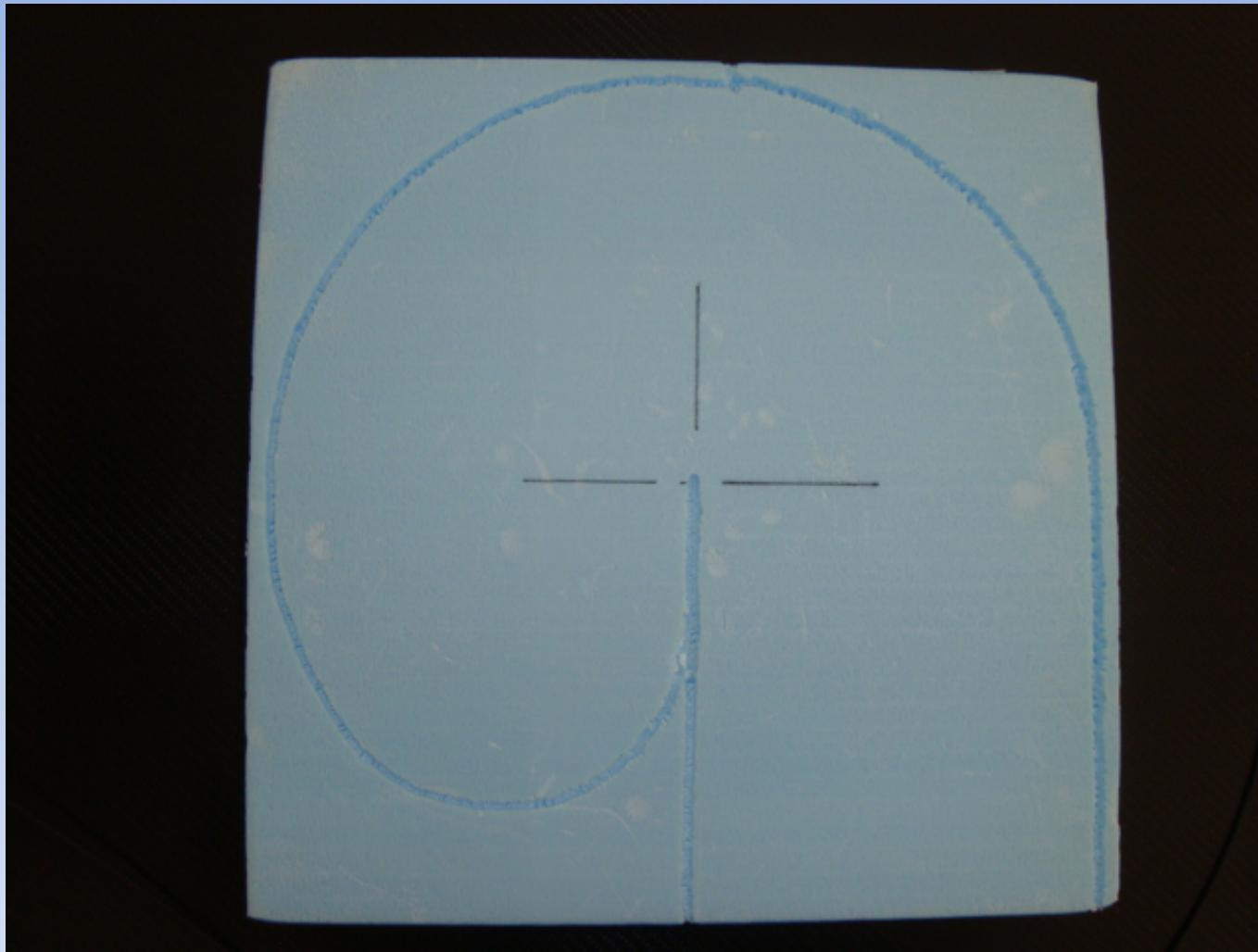
**Custom in-air calibration phantom for the W1 scintillator. The pattern on the vendor-supplied calibration phantom was transferred to a piece of Styrofoam and traced out with a drill bit.**
