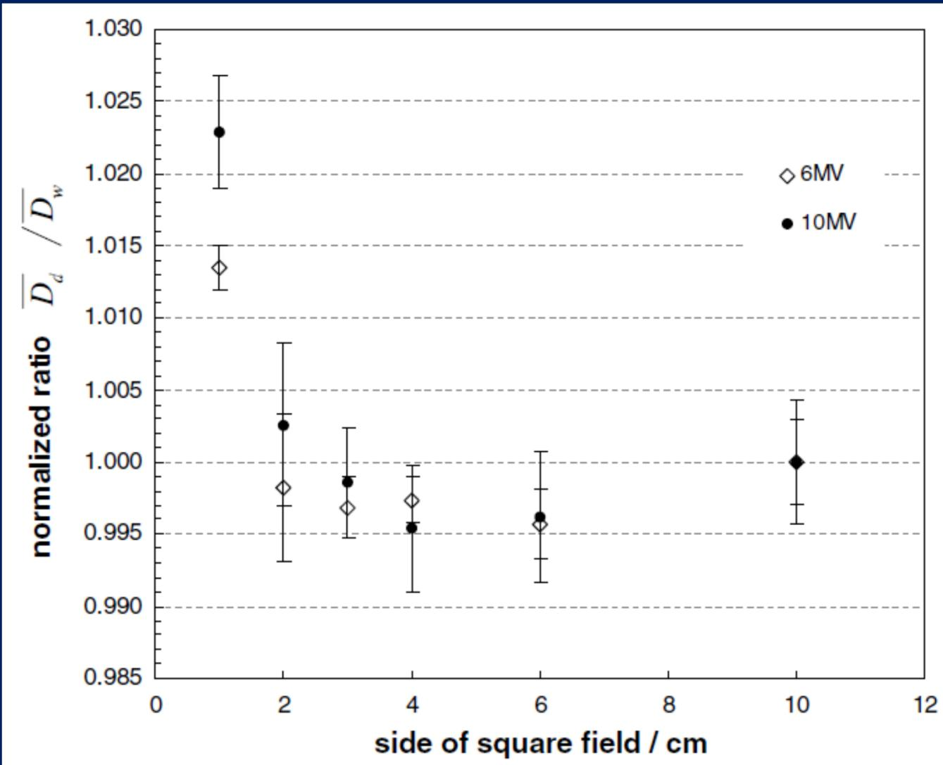
MC calculations of the field size dependence of the output factor for a diamond detector for 6 and 10 MV
