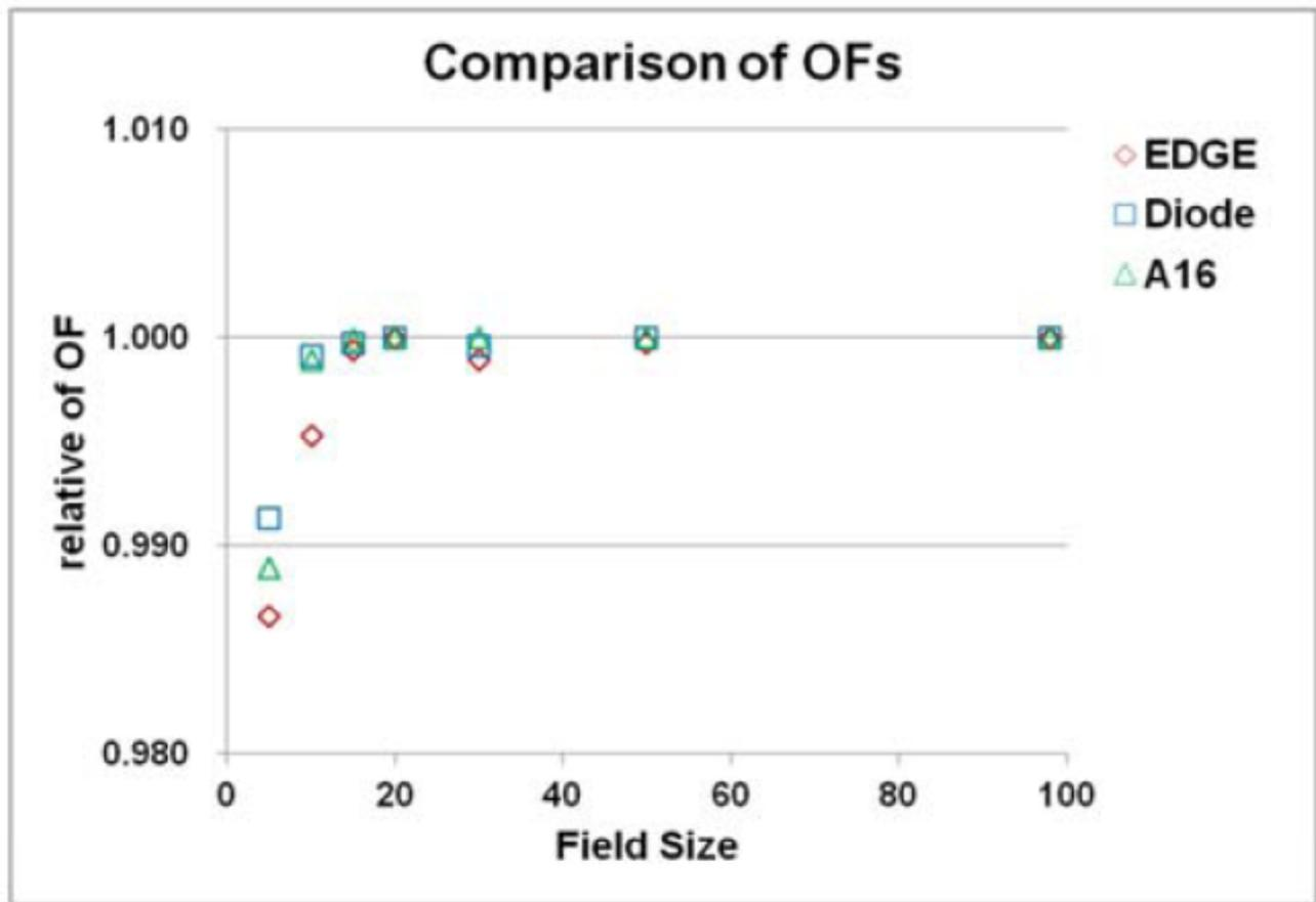
Measured relative output factors for 6 MV photons for various field sizes for the Edge, diode, and A16 detectors
