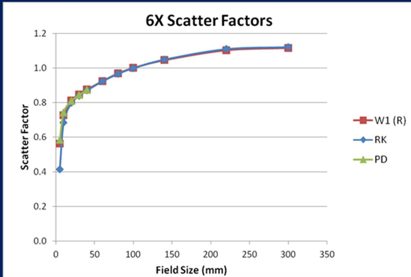
Scatter factors (Scp) for the 6X photon beam measured with the W1 scintillator, RK ionization chamber (RK) and electron diode
