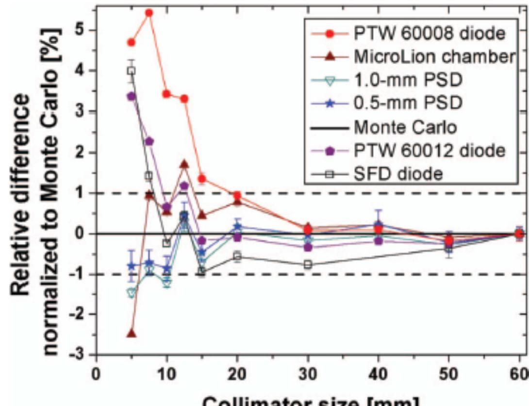
Relative total scatter factors normalized to MC calculations (solid black line) for various detectors
