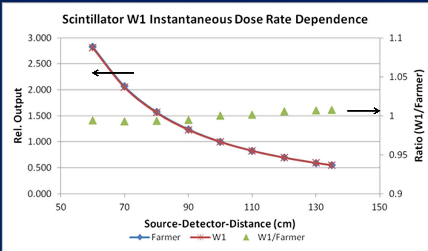
A Farmer ionization chamber which is known to have little instantaneous dose rate dependence was used as reference. For both detectors, the output was normalized to that of 100 cm SDD.
