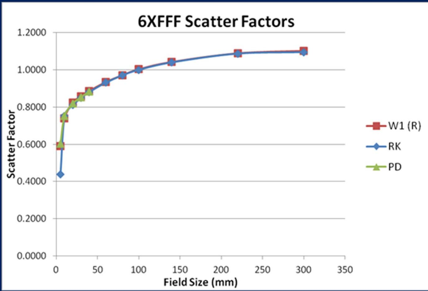
Scatter factors (Scp) for the 6XFFF photon beam measured with the W1 scintillator, RK ionization chamber (RK) and electron diode.
