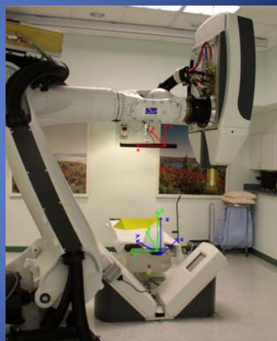
FIG. 3. The black isopost is mechanically mounted on the base frame of the imager system. The isocrystal at the tip of the post defines the coordinate system reference of the CyberKnife ® system. The robot is going through the path calibration process (Sec. III B 1), with the beam laser scanning the isocrystal.
