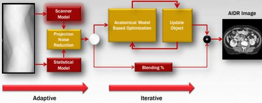
The scanner model analyzes the physical properties of the CT system at the time of the acquisition.
