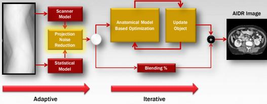
Adaptive processing in the raw domain based on the measured scanner and statistical modeling that reduces noise and artifacts.
