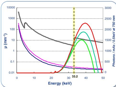
A high energy x-ray spectrum (mean energy above 33.2 keV – the K edge of iodine) is used to take advantage of the differential attenuation of iodine relative to the soft tissues.
