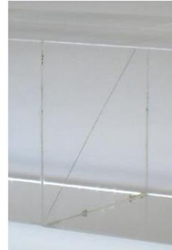
Slanted tungsten wire much smaller than the system point spread function (PSF)
