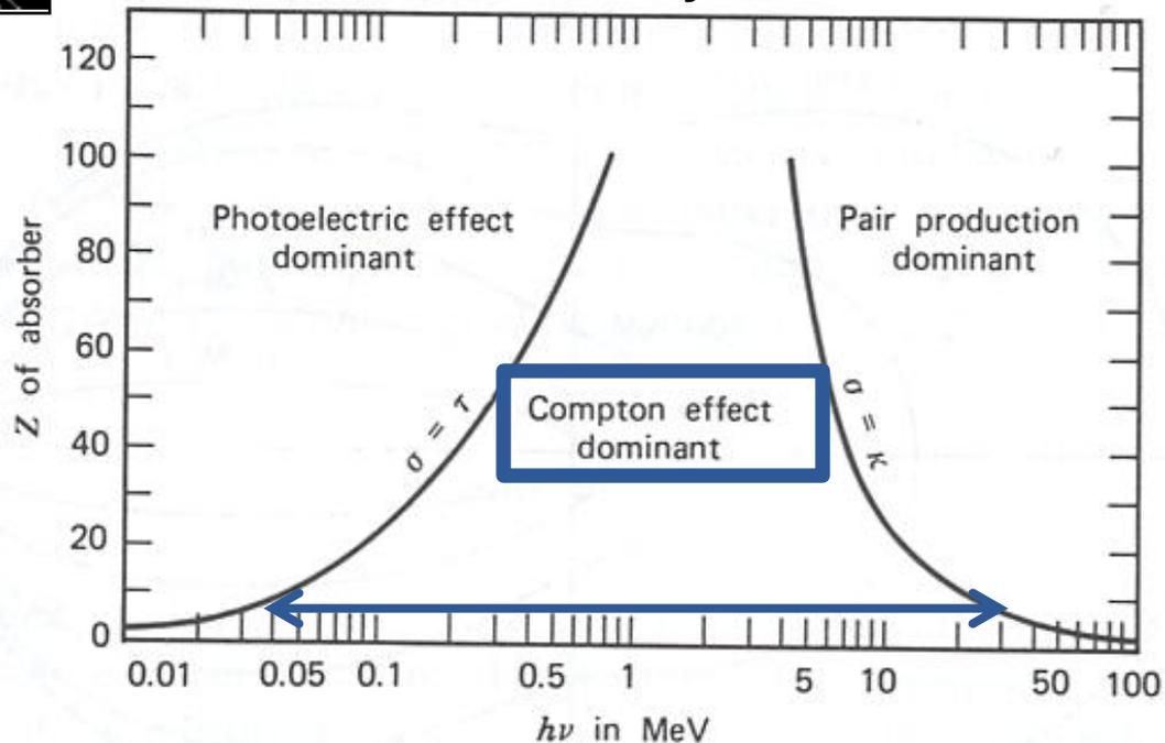
**Figure 2-20** The relative importance of the three major types of gamma-ray interaction. The lines show the values of  $Z$  and  $h\nu$  for which the two neighboring effects are just equal. (From *The Atomic Nucleus* by R. D. Evans. Copyright 1955 by the McGraw-Hill Book Company. Used with permission.)
