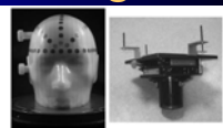
Figure 2. Stereotactic radiotherapy treatment delivery with excessive beam entrance positions as a function of acceleration and table rotation angles (left). The plate used in the centre (Case 2) to hold the cylindrical additional collimator (right).
