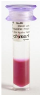
NIST traceable F-18 STD "S" vial geometry
