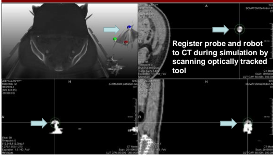
Guide probe placement towards non-interfering positions during simulation: probe placement map
