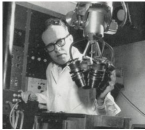
William Fry at the University of Illinois, Champaign, circa 1960, with a 4-beam high-intensity focused ultrasound applicator for neurosurgery.
