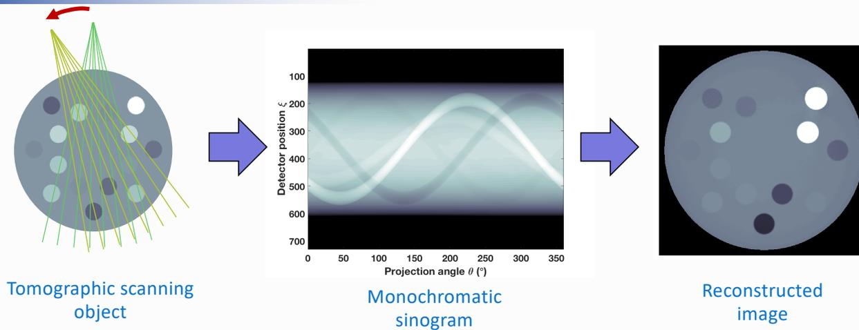
CT theory: the conversion of a 2D function into a sinogram representation is known as a *Radon transform* and its inverse operation often referred to as *Filtered Back Projection*
