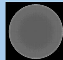
Example of BH artefact for a homogeneous cylindrical phantom
